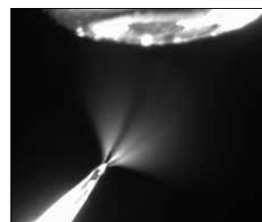
Split-Spray Spray voltage too high
