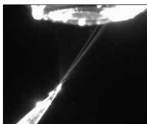
Jet Spray Spray voltage too low
