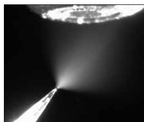
Perfect Plume Spray voltage is optimal
