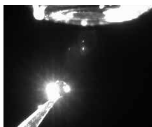
Droplet formation Spray voltage too low
