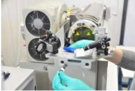
Figure 4.5 Remove the interlock pin cover before mounting the source to the source ring
