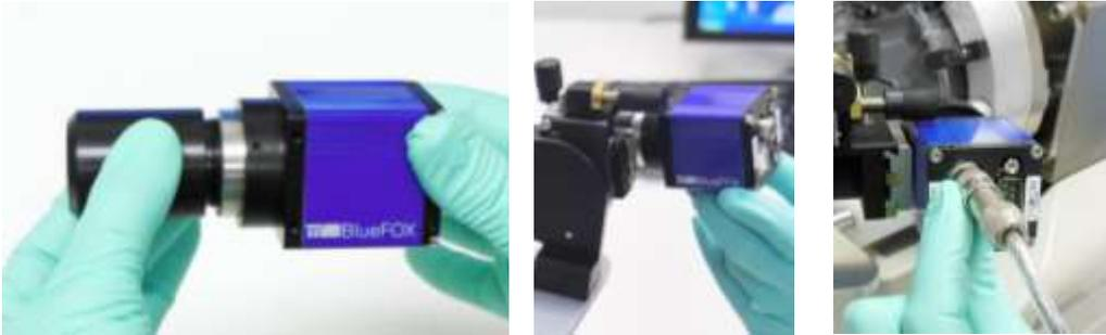
Figure 4.11 Attach the lens tube to the camera body (left). Orient camera as shown (center) and insert lens tube through camera mounting ring. Connect USB cable (right).
