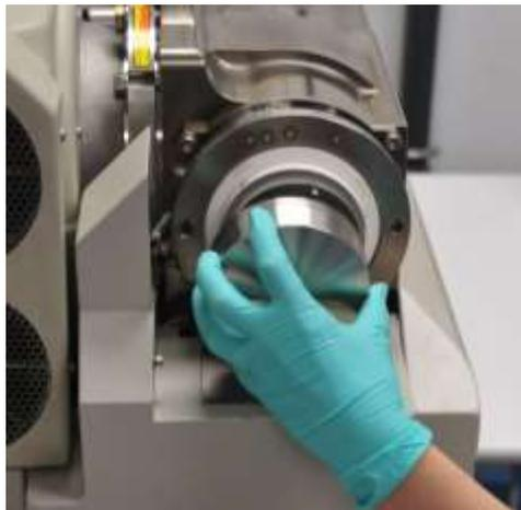
*Figure 4.1 Remove the standard curtain plate from the nanospray interface (4000 shown)*
