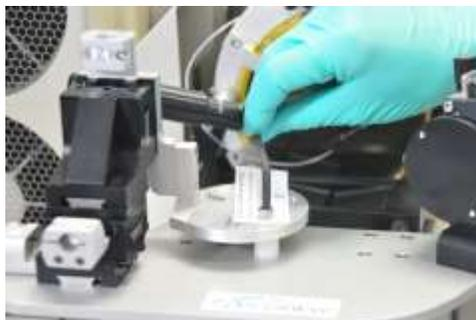
Figure 4.7 Remove the shipping bolt and tube
