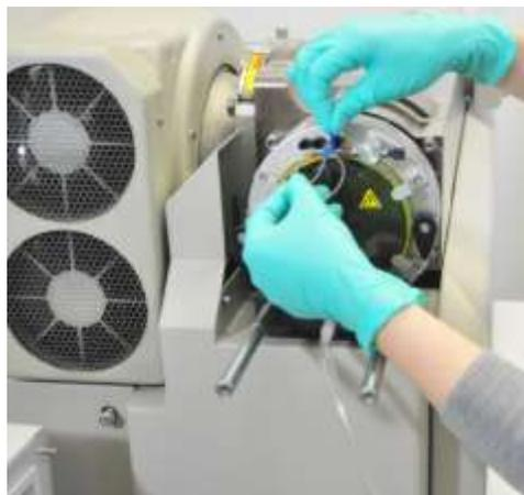
*Figure 4.4 Free the nebulizer gas tubing*
