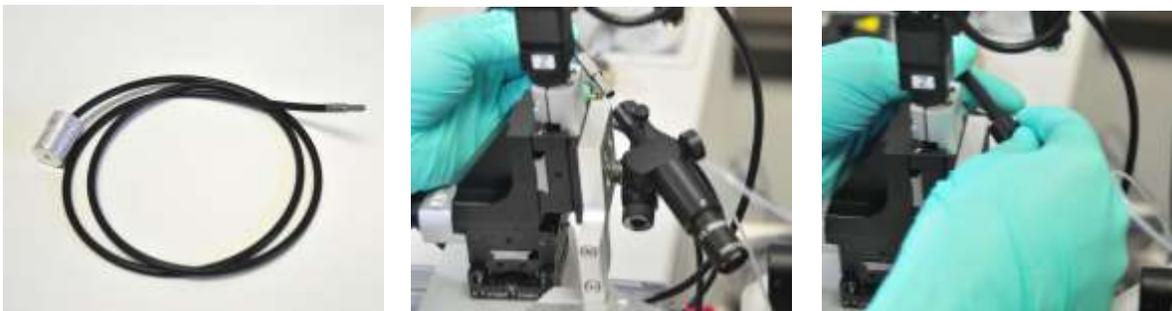
Figure 4.12 Fiber optic cable (left); Insert fiber optic into the illuminator mount on Digital PicoView (center); Tighten thumb screw to secure fiber optic in place (right)
