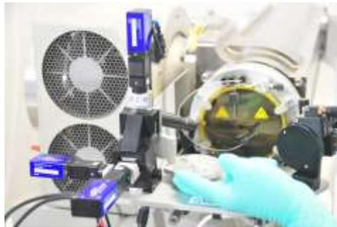
*Figure 4.9 All three stage actuators installed*
