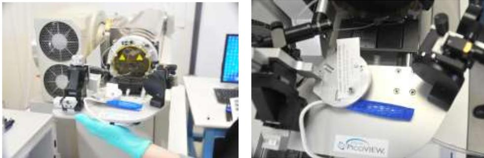
Figure 4.6 Slide the source onto the source ring rails. Push source as far forward as possible.
