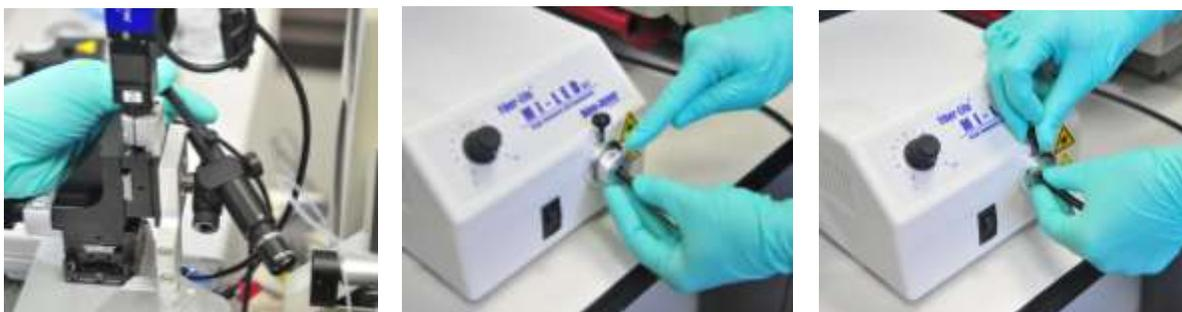
Figure 4.13 Fiber optic cable installed in illuminator mount (left); Insert fiber optic coupler into illuminator (center); Tighten the thumb screw to secure the coupler in place (right)
