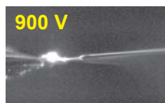
900 V Spindle Mode Pulsed Spray +Large (5 µm) Drops
