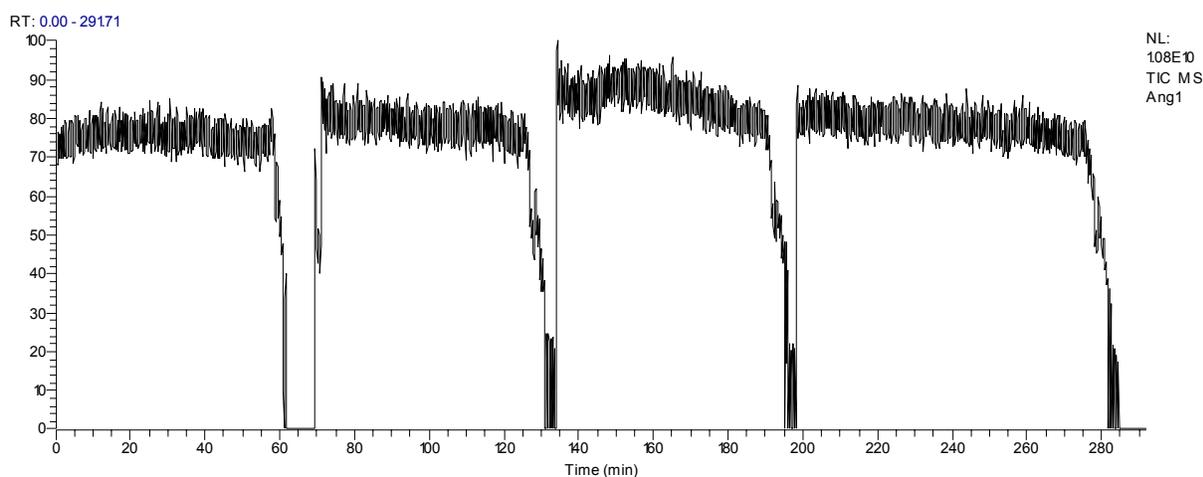
Figure 2 - Total ion chromatogram of Angiotensin I from an offline nanospray emitter with a reactive platinum coating.
