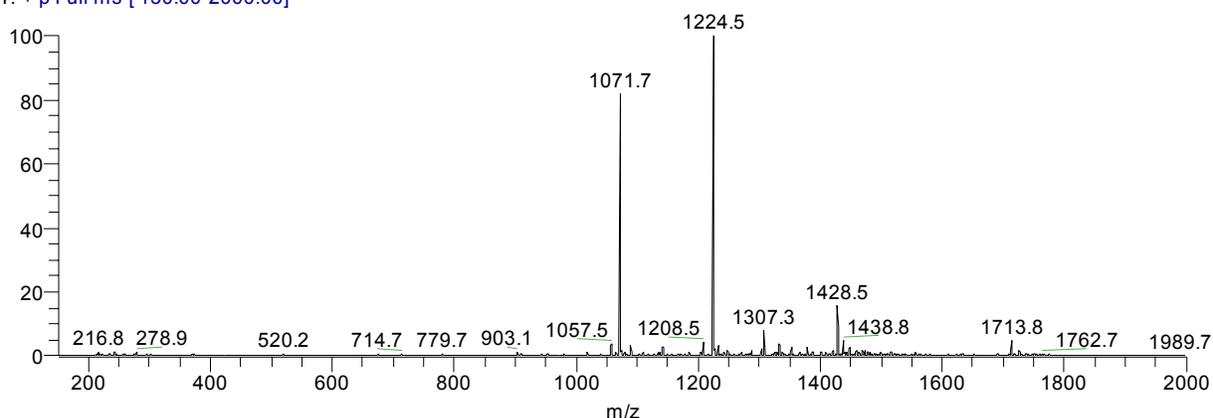
Figure 1 – Mass spectrum of a 10  $\mu\text{M}$  Ubiquitin solution produced with a Pt/SiO<sub>2</sub> multilayered emitter with over 830 hours of service. The mass spectrum was acquired by a Thermo Finnigan LCQ<sup>Deca</sup> equipped with a PicoView nanospray source.
