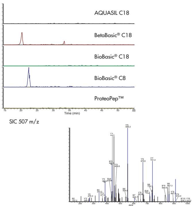
Figure 7 - Base peak reconstructed ion chromatogram for  $m/z$  507 ( $M+2H$ )+2 of a trypsin digest mixture on a ProteoPep™ PicoFrit™ column incorporated with five different sample trap materials (top).
