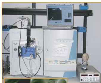
A Figure 1 - (A) System configuration on an LCQ Deca™ (Thermo Electron) (B) Schematic of the spray analysis and orthogonal control system
