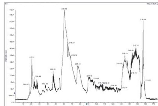
Even with a 4-fold sample dilution, the 75  $\mu$ m ID column exhibits sample overload
