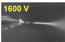
Figure 4 - Scattered light images for commonly observed spray modes. The applied voltage is on the upper left hand corner of the image. The emitter was 15 \mu\text{m} and the mobile phase was 50% MeOH, 1% acetic acid pumped at 250 nL/min. the automated control system is designed to achieve a stable-cone jet mode under any condition.
