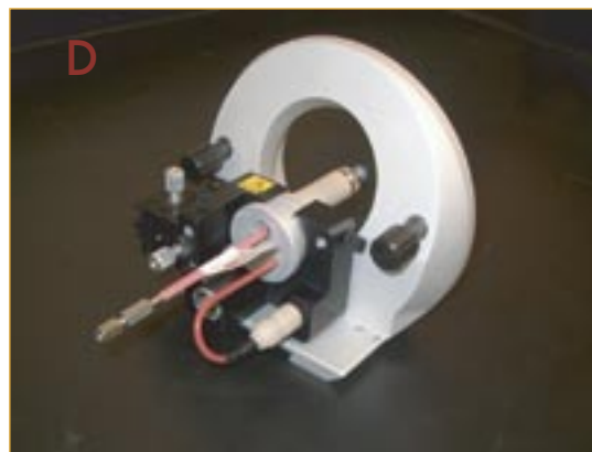
(C) Photo of PicoView® 150 nanospray source on LCQ Deca™ (D) Photo of Thermo Finnigan™ nanospray source with integrated grounding and HV junction used for capillary column experiments on the LCQ Deca Plus™
