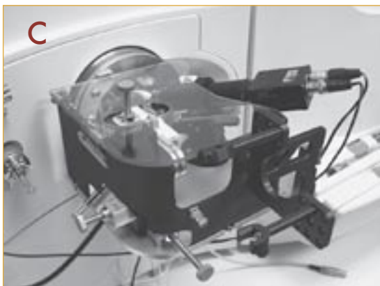
(C) Photo of PicoView® 150 nanospray source on LCQ Deca™ (D) Photo of Thermo Finnigan™ nanospray source with integrated grounding and HV junction used for capillary column experiments on the LCQ Deca Plus™
