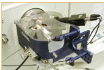
Figure 1A PicoView® 150 on a Thermo Finnigan™ LCQ Deca™
