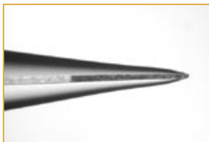
Figure 1B Integral frit and emitter of a PicoFrit® C18 column
