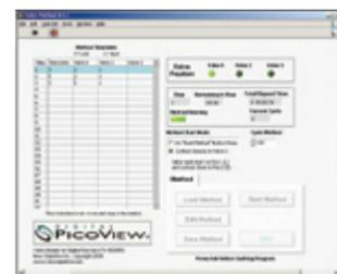
**Figure 7** Valve Method™ Module. Valve state and time values are used to actuate valves during a run. The valve module can either generate a of a valve switch or wait for a contact closure for control by another instrument. Here is shown the use of the valve module to control two valves for trapped sample injection using a valve mounted on the source, rather than the valve on the autosampler to reduce system volume.
