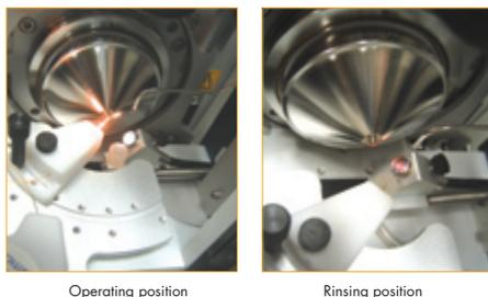
**Figure 3** Digital Divert™ program provides automated emitter rinsing between sample runs. Both the emitter and LTQ™ inlet remain clean by eliminating build-up of salts, etc.
