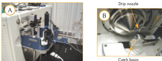
**Figure 2** A) Source mounted on LTQ™. B) Detail of emitter rinsing station.
