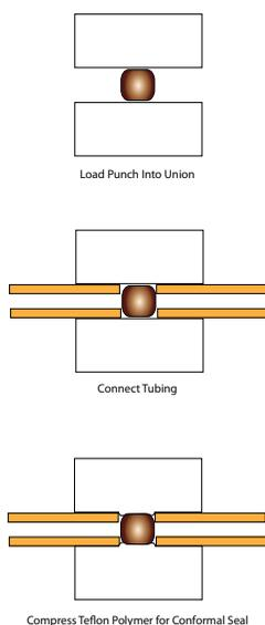
**Figure 2** Segmented flow extraction from the punch
