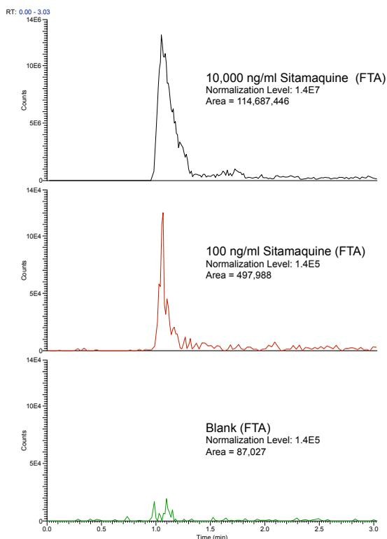
Ion trap based SRM elution profiles at two different analyte concentrations and a blank. The segmented elution enables a tight elution profile preserving high sensitivity and signal-to-background ratio. Elution is rapid, with an MS cycle time of better than 2 minutes.
