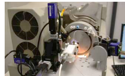
DPV-450 Digital PicoView nanospray source installed on the AB SCIEX 4000 Q TRAP
