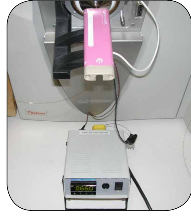
Heated PicoChip column with the Omega Benchtop controller
