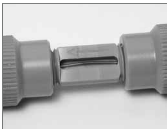
FIGURE 10 A slight bend in the installed column indicate may be visible and is indicative of a successful seal
