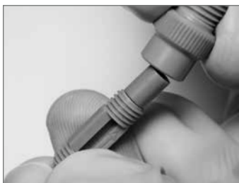
FIGURE 6 Set the capsule union on the inlet end of the column holder. Cover with an end cap and tighten only until the threads are engaged.
