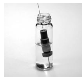
FIGURE 8 Column tip pulled back into sleeve
