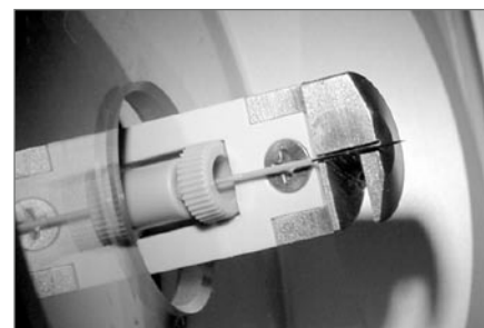
FIGURE 1 MicroTight® union holding a standard-length PicoTip® emitter
