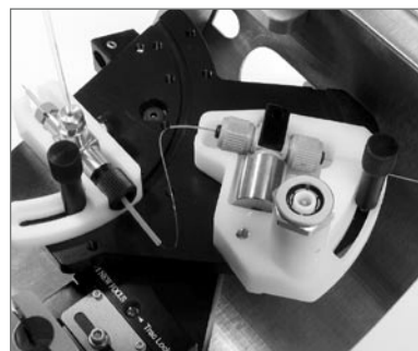
Sheath gas module in use on a PicoView® Model PV-300 with the uncoated tip module
