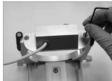
Figure 4A: Removing one of the 6-32 x 5/16" flat head screw securing the electronics housing assembly onto the interface flange
