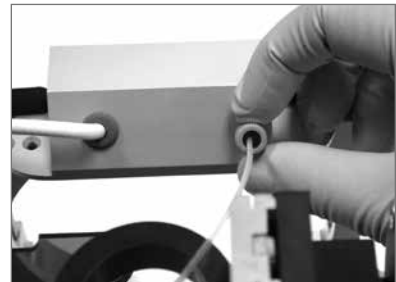
Figure 18C: Inserting the sheath gas tubing into the sheath gas port on the sheath gas enabled electronics housing assembly
