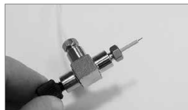
Figure 9: The tip of the emitter protrudes 0.5 to 2.0 mm past the PEEK sheath nozzle
